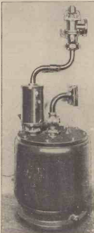
The first carburettor for the vaporisation of petroleum fuels. It was made by Benz, in Germany, about 1886, and was used for gas engines.
