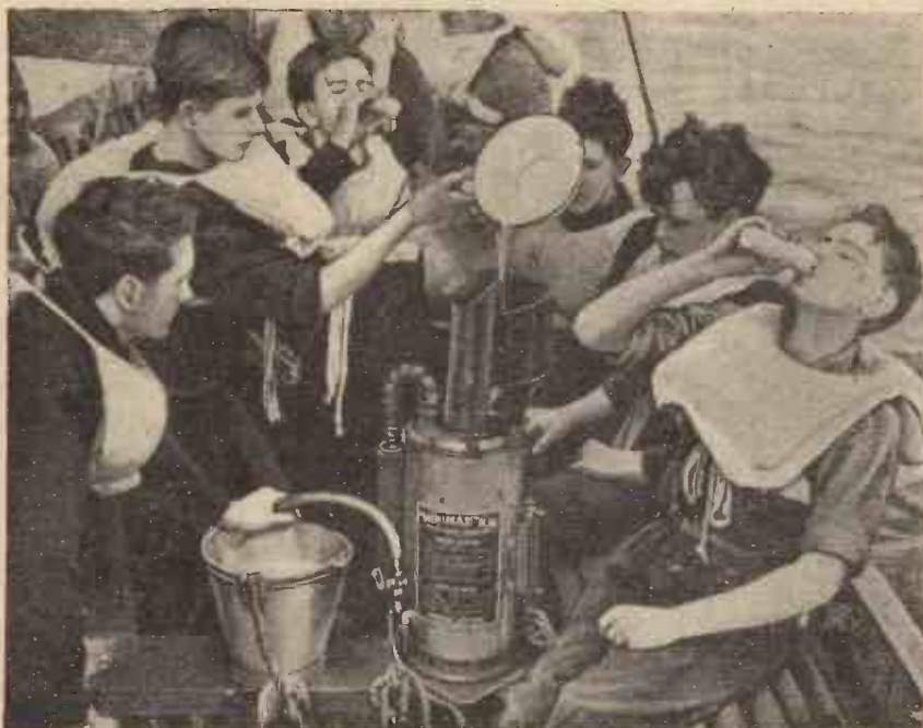
A test being made under shipwreck conditions with the Minimax Fresh Water Producer. (By courtesy of Minimax, Ltd., and The Sphere.)
