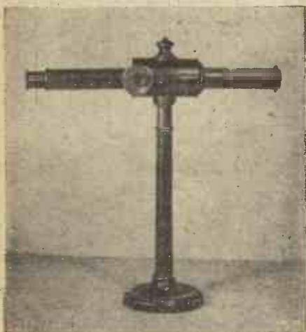
A spectroscope of Brewster's day (1830). It was by means of an instrument of this nature that he discovered the "absorption bands" of the spectrum.
