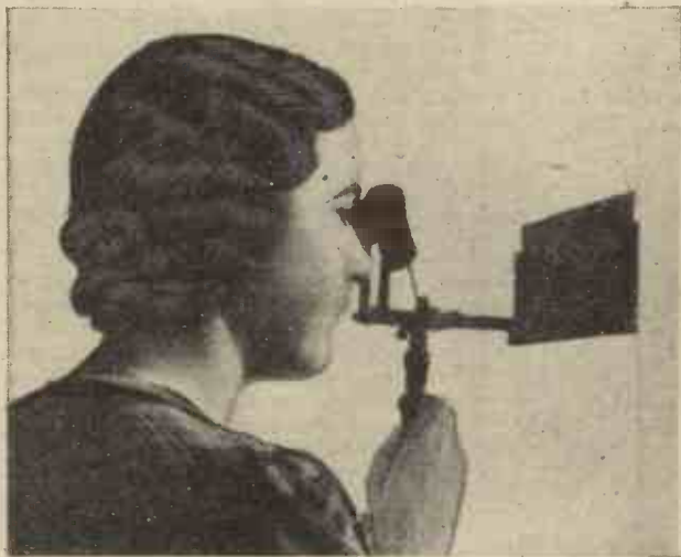
The modern version of the Brewster lens-stereoscope—an instrument which is light, portable, and which folds up when not in use.
