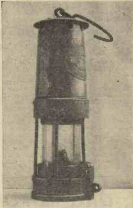
The miner's lamp, an indispensable aid to coal-mining. It is based on the simple principle illustrated in the diagrams given below.
