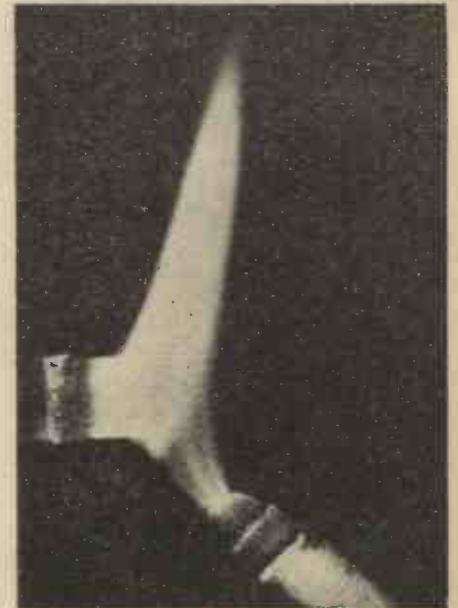
"Electrical flame"—a photograph of the flame of white-hot, glowing carbon vapour existing between the carbon electrodes of a high-power arc lamp.
