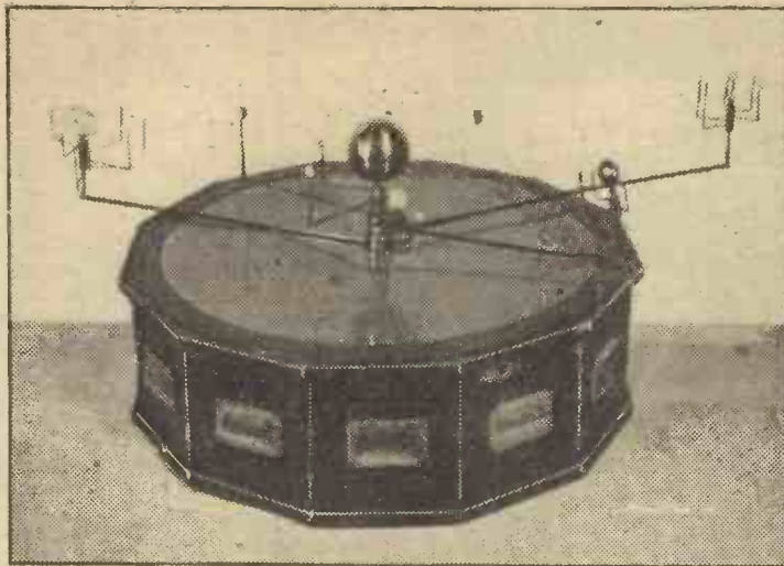
A planetarium or orrery. Such a device produces a mechanical representation of the motions of the heavenly bodies. The orrery here illustrated was constructed shortly after Graham's death.
