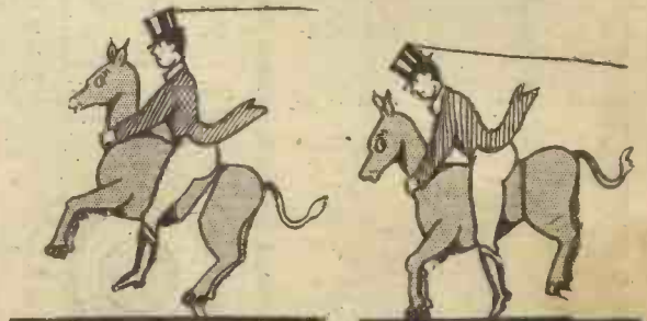
Figs. 41 and 42.—The galloping ass, the hindquarters of which are hinged. The action of pulling on the cord attached to the hat supplies the motion.
