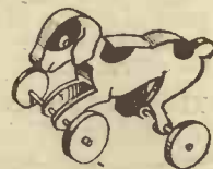
Fig. 36.—A leaping dog novelty. The spindles pass through the wheels eccentrically.
