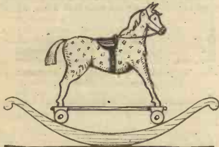
Fig. 37.—A novel rocking motion device in which the horse travels forward and appears to vault.
