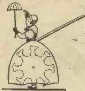
Fig. 43.—A simple idea for making a walking doll. When the doll is pushed along by means of the handle, the action of walking is imitated.
