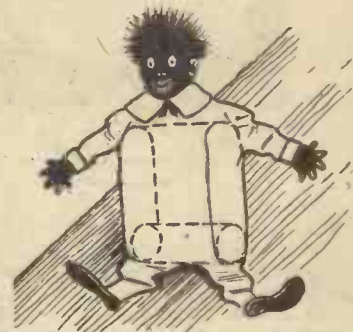
Fig. 49.—Squeaking toys can be made by placing a small bellows weighted with lead inside them.
