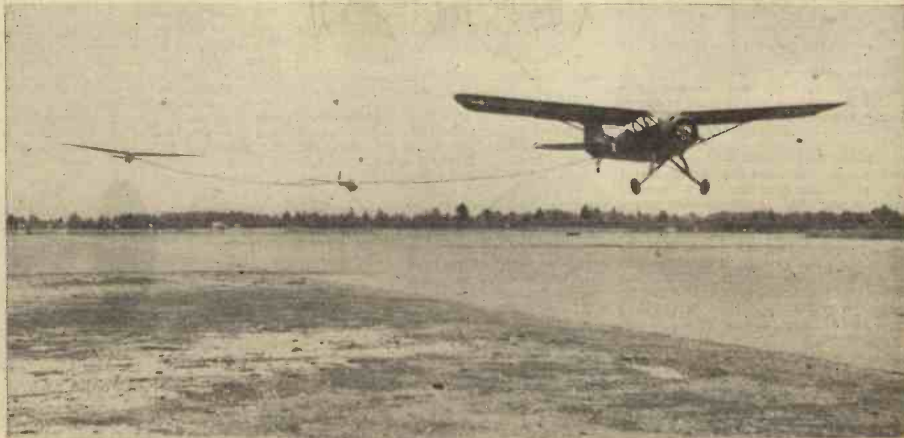
Glider leave the ground before their towing plane, and here, at the U.S. Army Air Forces' Glider School at Elmira, New York, they are clear of the ground, riding higher than the plane. They take-off after a run of about 500 feet while a tow-plane needs a run of about 1,000 feet. In flight the gliders remain slightly above the level of the tow-plane, with nose a little down to maintain lift.
