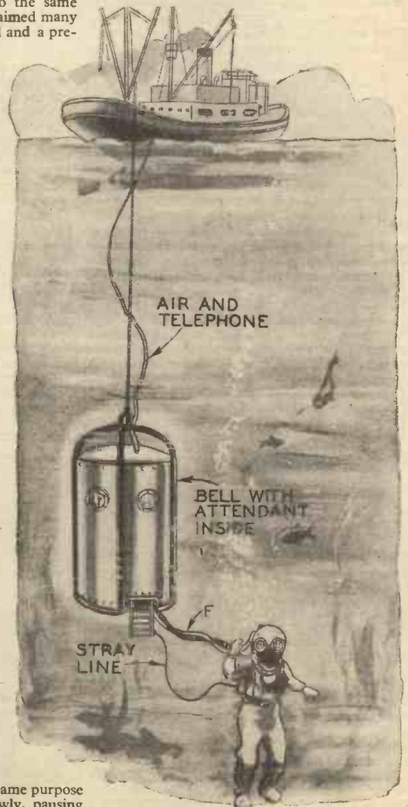
Showing how deep-sea diving is carried out by the diver from a diving bell.
