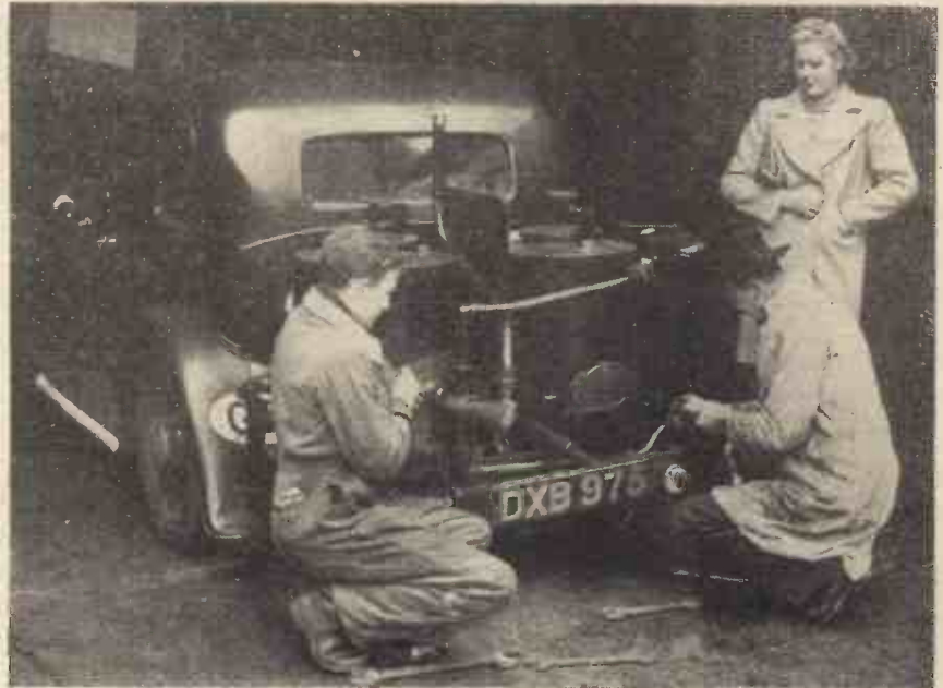
Fitting a gas-producing unit to a 10 h.p. car. The complete unit, including fuel, weighs 2½ cwt.
