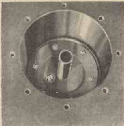
Fig. 4.—Interior of pressure chamber showing gland leather, oil conduit, and retaining ring for gland leather.
