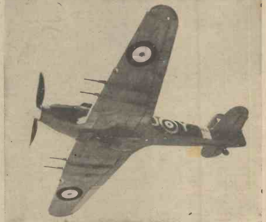
The Hurricane II, with improved armament consisting of 20 mm. cannon the combined fire of which is 2,400 shells per minute
