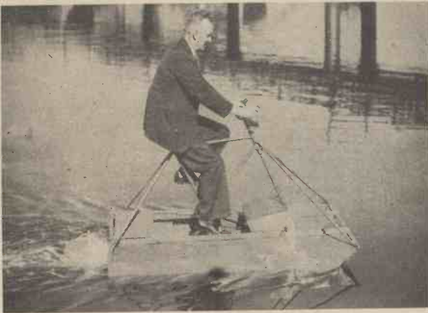
This water-cycle, constructed by J. Atkinson, of Sydney, Australia, is constructed with a bicycle frame, two pontoons, and a special geared drive for the propeller. The machine is capable of 8 knots.
