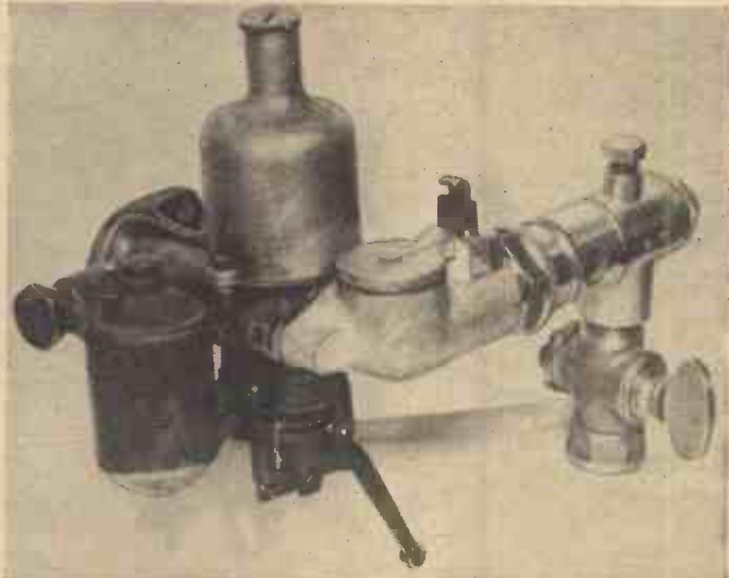
Fig. 4. Gas carburettor showing method of fixing to the S.U. petrol carburettor. The air flap is in the closed position for running on gas
