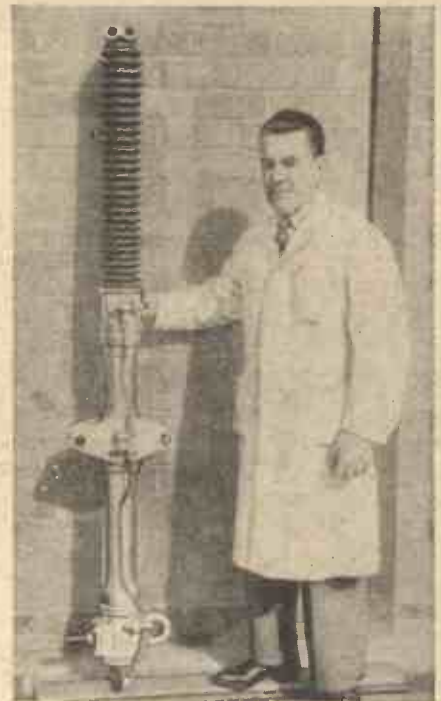
Fig. 6. A Lockheed hydraulic jack, specially designed for operating the retractable undercarriage of the Armstrong Whitworth Imperial Airways "Ensign" air liner.
