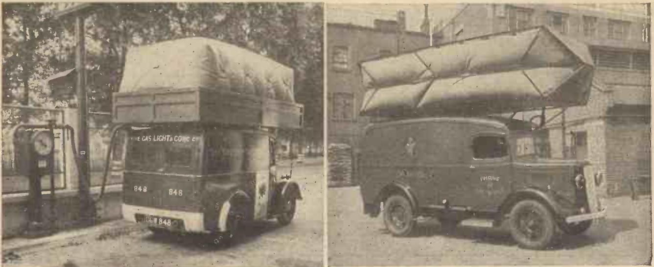
Figs. 1 and 2. (Left) A van with a box crate. (Right) A van fitted with a Walsh collapsible crate.
