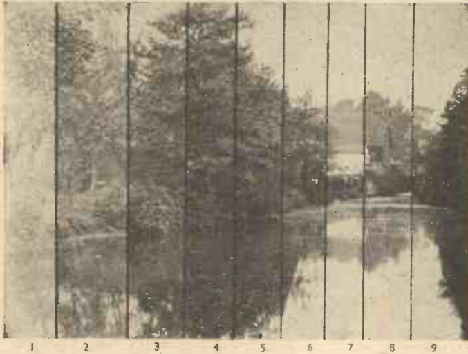
Showing how nine test exposures can be obtained on one piece of paper.
