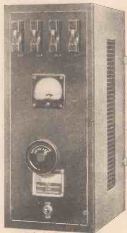
Fig. 10. A standard selenium-type rectifier as used for trickle charging.
