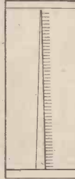
Fig. 7.—A gauge for reading the size of the hour wheel socket or cannon pinion. It is similar to a pivot or mainspring gauge.
