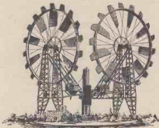
Proposed design of wind generator: driving wheels would be 1,000 ft. in diameter.
