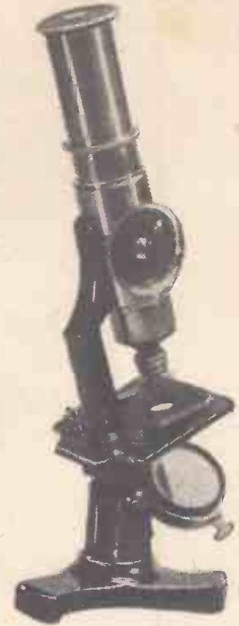
An ordinary optical microscope of a simple amateur type. With this instrument a magnification of about 200 times can be obtained
