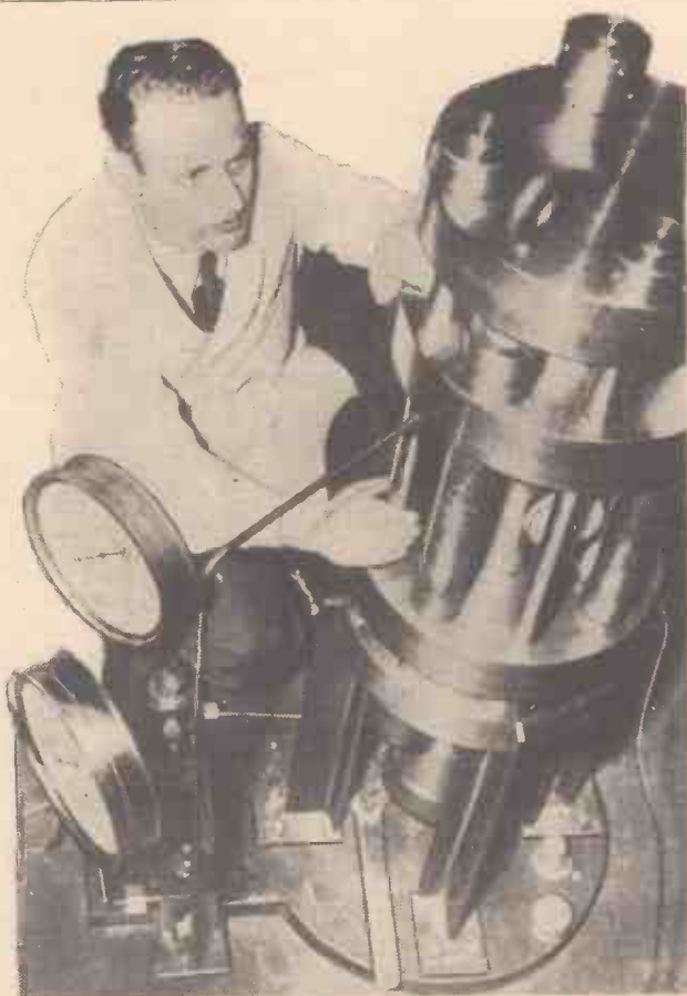
Dr. R. Goranson, of Washington, D.C., with his "cascade bomb" with which he has created a pressure of 3,000,000 lb. per sq. in., claimed to be the greatest pressure ever to be created by machine. This feat was accomplished at the Geophysical Laboratories of the Carnegie Institute.
