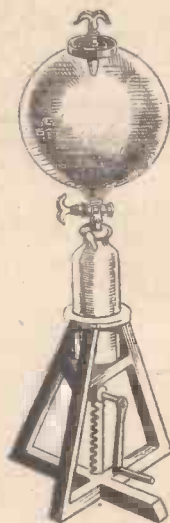
Boyle's original air-pump, the first mechanical air-pump to be made in this country. With his pump he made a large number of experiments upon the physical nature and properties of air
