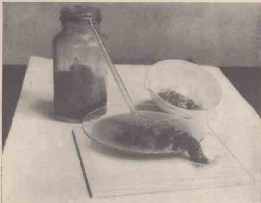
A quantity of soap made from kitchen grease. The soap is shown "in the crude," i.e. before pressing and refining
