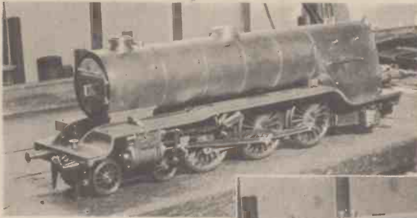
Fig. 28.—The finished outer boiler casing in position on the chassis
