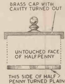
Fig. 9.—A brass cap hollowed out to fit tightly over the halfpenny
