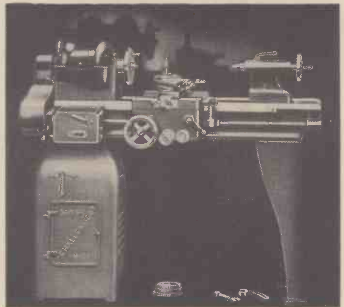
A fine example of a modern back-gear screw-cutting lathe, made by B. Elliott and Co., Ltd.
