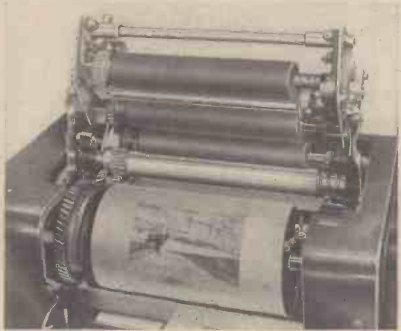
(Right) The automatic printing and duplicating machine. (Left) The double inking unit
