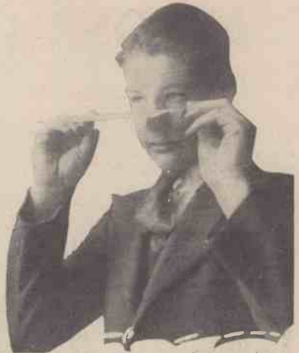
By holding up a sheet of paper to eye level and glancing along it, the presence of invisible ink writing may nearly always be detected
