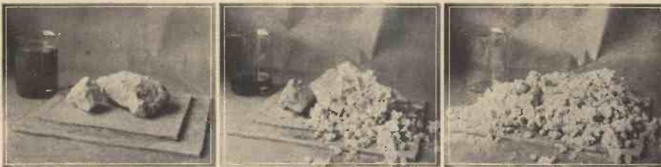
A series showing the conversion of an oxide to a hydroxide by mere addition of water. (Left) Lumps of quicklime calcium oxide, \text{CaO} . (Centre) The quicklime has partially combined with the water which has been added to it, the effect being known as the "slaking" of lime. (Right) Here the quicklime has been wholly converted into slaked lime, or calcium hydroxide, \text{Ca(OH)}_2 . Note the great increase in volume of the material after the water absorption.
