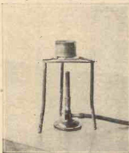
Preparing copper oxide by heating copper nitrate.
