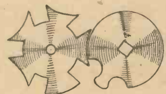
Figs. 3 and 4.—(Left) A new hook before being cut off. (Right) A stop-work mechanism.
