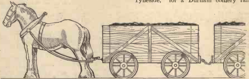
The earliest form of truck haulage was done by horses which pulled a truck along a wooden-railed tramway.
