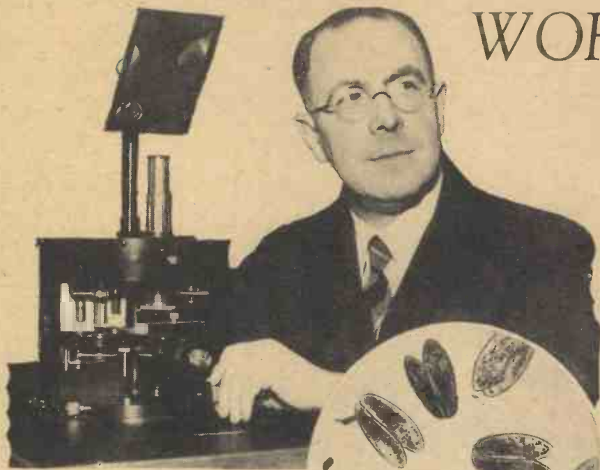
One of the 12 microscope reflector units in the Microvivarium exhibit. On screens 5 ft. in diameter, images of one-cell animals, whose whole world is a drop of water, will be magnified 2,000 times in their actual colours. (Inset) a magnified view of a group of one-cell animals.
