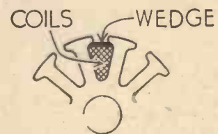
Fig. 8.—An armature with semi-enclosed slots.
