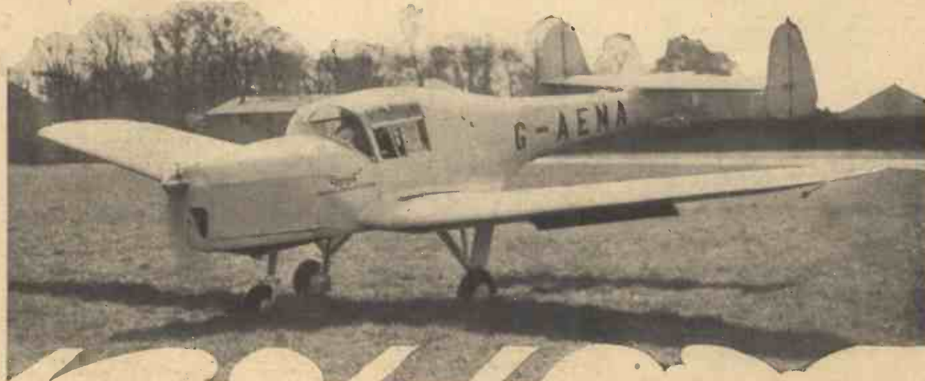
A new type of training machine for air pilots known as the "Cygnet," landing during a recent demonstration at Hanworth. It is one of the first British single-engined machine to be fitted with double rudders and fins.
