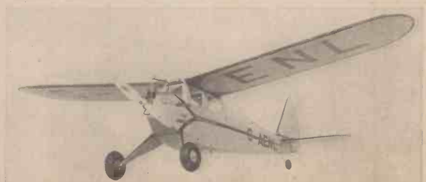
The "Privateer Junior" also supplied by the Model Shop. It has a 4 ft. 6 in. wing span and is powered by a Trojan engine.
