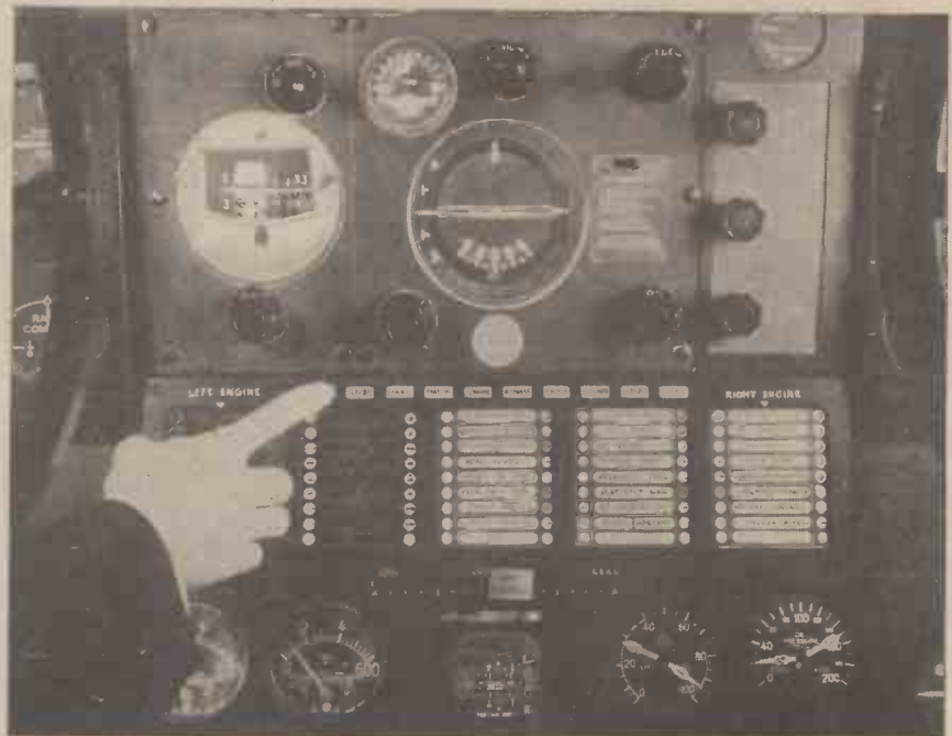
To simplify the pilot's operation of the 'plane engineers have developed the above pictured "telltale" device which automatically checks the functioning of all instruments and vital parts of the 'plane, and, supplementing the so-called Sperry "automatic pilot," is virtually a "fourth pilot." Experts say it decreases "pilot fatigue" and hence increases air line safety.
