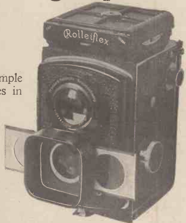
Fig. 1.—A Rolleiflex camera fitted with a home-made sliding filter holder, and gelatine filters.
