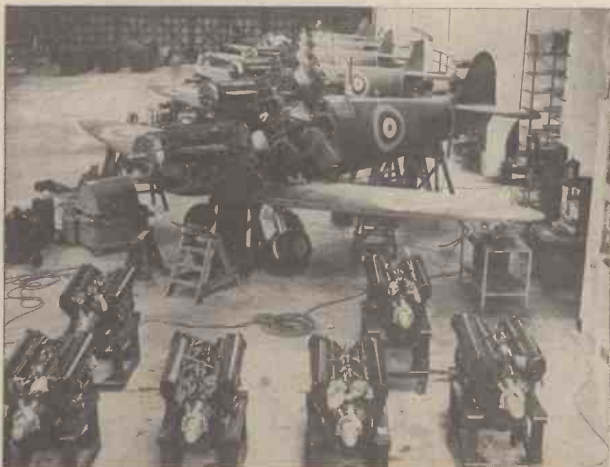
A view of Spitfires being assembled in one of the shops at Eastleigh. In the foreground are Merlin II engines waiting to be installed.
