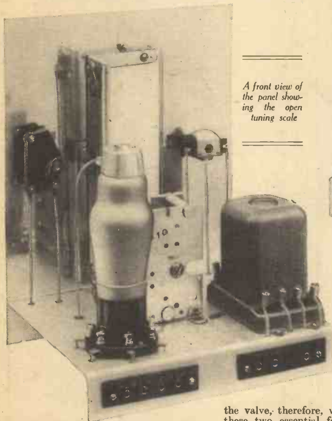
This three-quarter rear view of the "P.M." One-valver shows the business-like layout which is adopted
