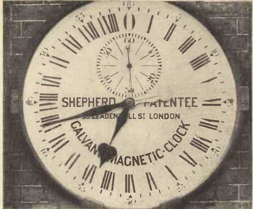
The twenty-four hours clock. This clock dial, which is mounted on the exterior side of the wall near the main entrance to the Observatory, is electrically connected with the Mean Time Clock. It indicates the time which has elapsed since the previous midnight. The photograph shows the clock indicating 13 hours 42 minutes 29 seconds, i.e. nearly 17 minutes to 2 p.m.
