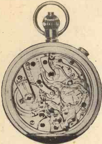
The split-seconds mechanism of a high-grade chronograph.
