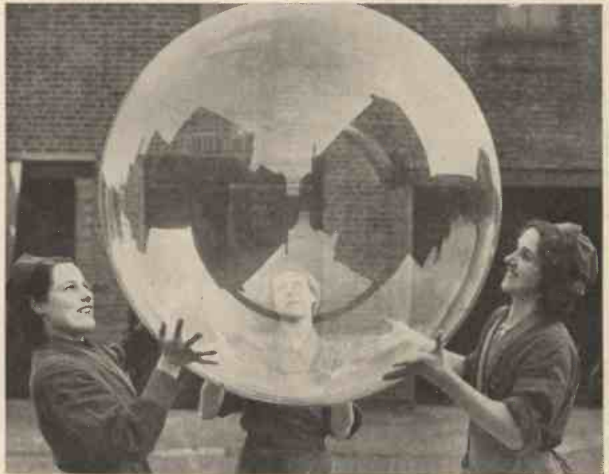
This is claimed to be the largest transparent ball ever made. It is produced from Perspex synthetic resin, a product of I.C.I., shaped by the Triplex Safety Glass Co., Ltd., and it was shown at the stand of Mouldrite, Ltd., at the British Industries Fair at Olympia. A feature of the ball is its high light transmission, and it can be looked through from any angle without the slightest distortion.
