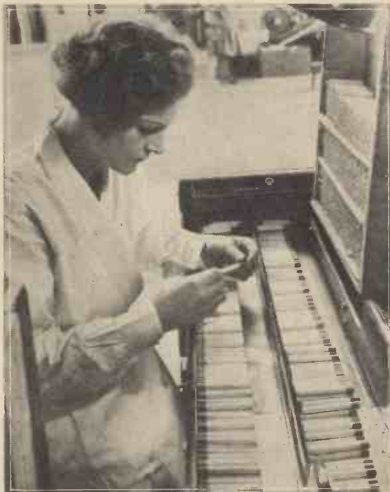
At every stage in the manufacture the cigarettes are subjected to the most rigorous system of checking. This work is done by girls who are specially trained so that they can see even the slightest fault at a glance. The picture shows one of the girls working on the final inspection.
