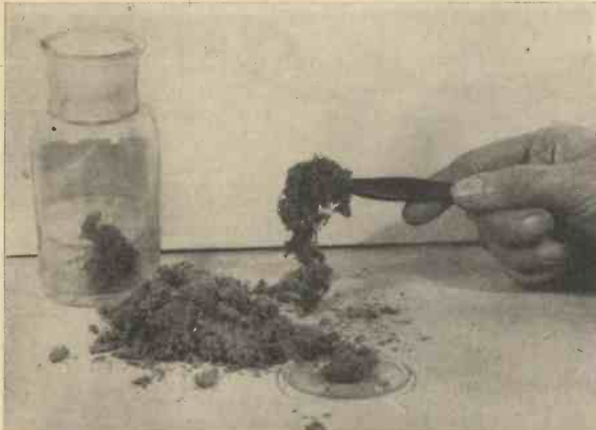
Platinised asbestos—a well-known catalytic agent. It consists of asbestos fibre impregnated with metallic platinum.
