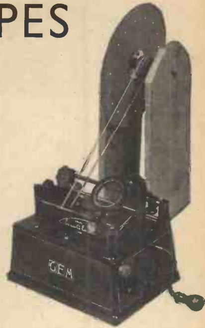
An old Edison phonograph utilised for the purpose of rotating a disc stroboscope. Time control of the revolution speed of the disc can be obtained in this way.
