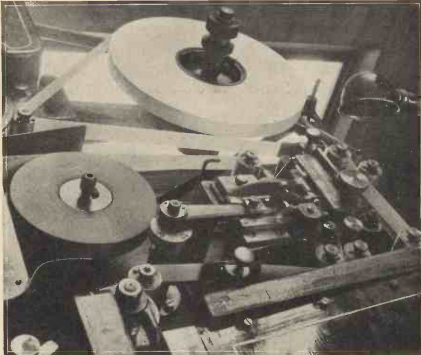
The cigarettes are rolled by a machine that holds over three miles of paper at a time—enough for 60,000 cigarettes. This machine also tips the cigarettes with cork. The cork arrives at the factory already wound in spools, one of which is seen on the left of the picture.
