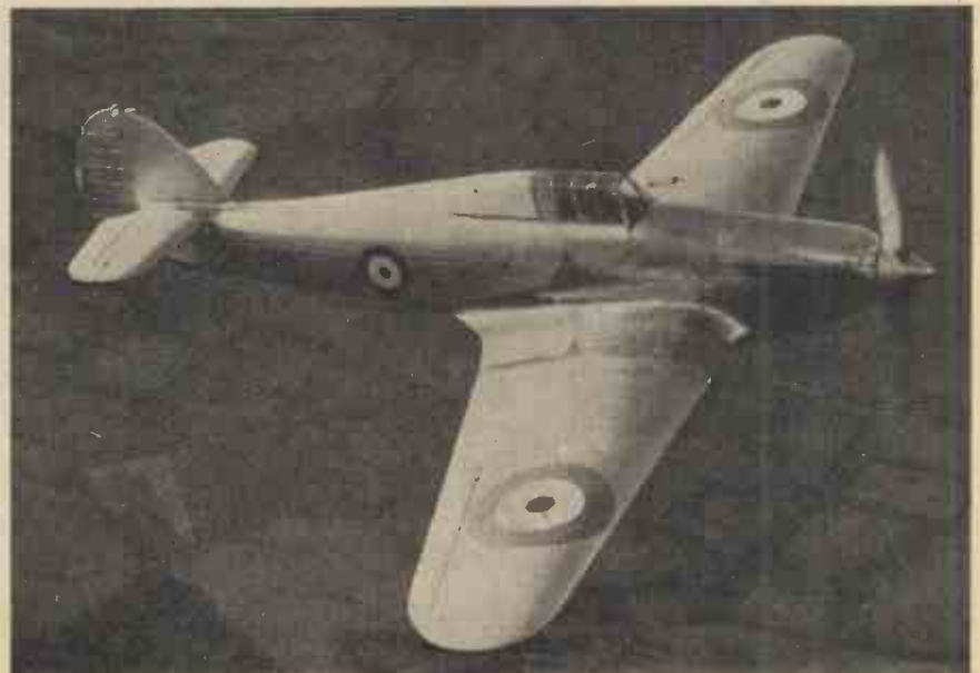
A Hawker Hurricane monoplane, the world's fastest machine, in flight. It has reached a speed of 443 m.p.h.
