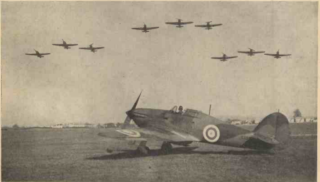
"Hawker-Hurricane" single-seater fighters, capable of speeds in excess of 400 m.p.h. They are low-winged, streamlined monoplanes, and the fastest military aircraft in the world. The illustration shows a squadron in flight and one of the machines on the ground.
