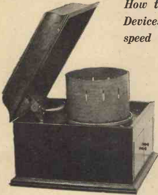
An illustration of the easily made "gramophone stroboscope."
