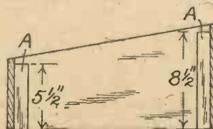
Fig. 11.—Section, showing the corner strengthening pieces.
