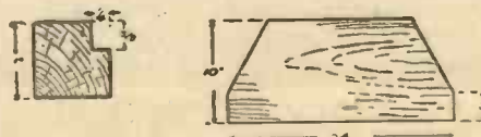
Fig. 16.—Section of timbers for window frame (left), and shape of wheel-arch panel (right).
