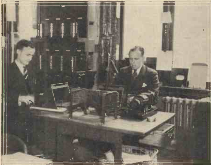
Transmission of messages by the "ticker." The subscriber receives the message almost simultaneously on his machine at the other end of the wire.
