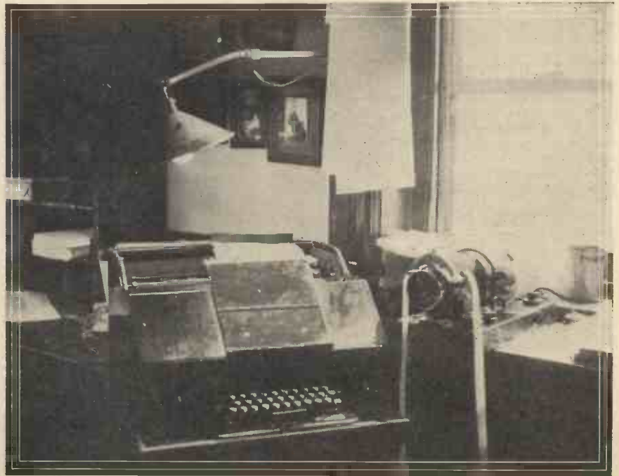
A wonderful machine—the automatic typewriter. The narrow tape which has been used earlier to send news to subscribers by means of the "ticker" is used again to operate the automatic typewriter, which cuts a stencil to be used in the duplicating machine. The sheets are sent out by hand in confirmation of the earlier messages.
