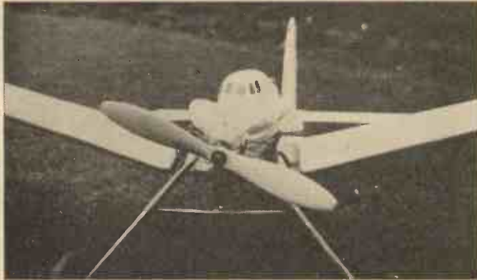
Fig. 24.—The nose and fuselage, showing the cabin and dummy engine fairings to strengthen the nose where the low-wing "cutaway" is situated.
