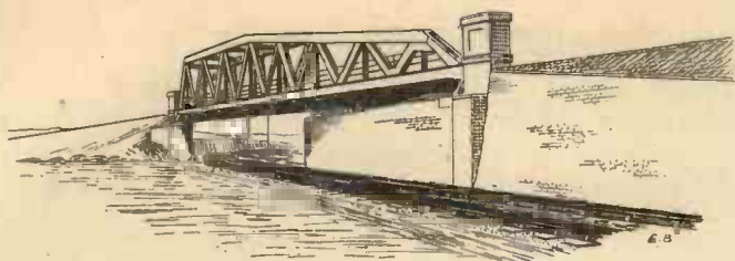
Fig. 7.—A girder bridge for a flying-junction.
