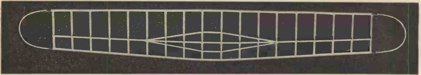
View of the uncovered wing, showing the swept-back leading edge.
