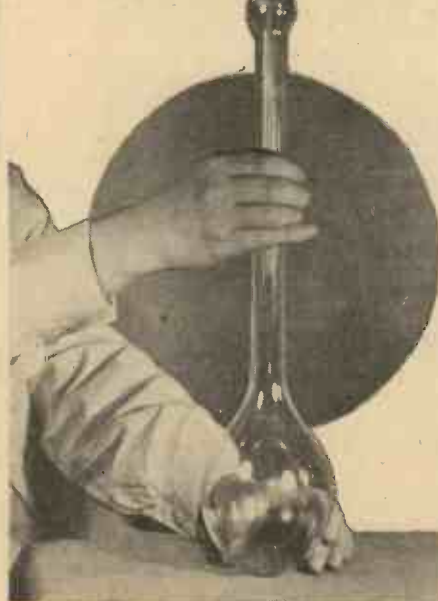
A bottle of neon. Although the gas is invisible and weighs but little, it is a most precious commodity. The quantity of neon in the bottle shown is sufficient to fill several large signs.
