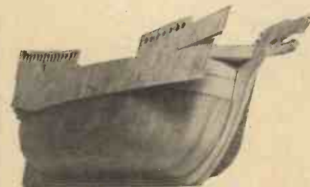
Fig. 6.—Fitting the bulwark into place. Note how the cut at the bow enables it to fit against the forecastle and hull.
