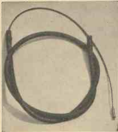
Fig. 6.—For light work, an old speedometer driving shaft may be used.
