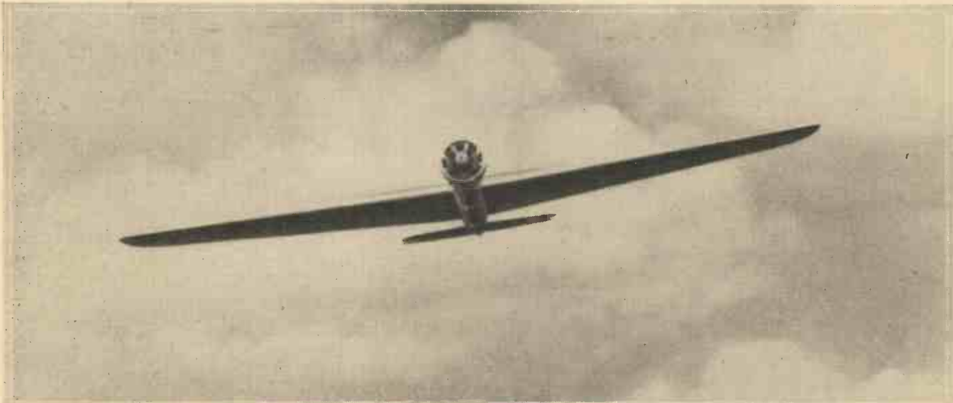
The Vickers "Wellesley" monoplane fitted with a Pegasus air-cooled engine. An order has been placed by the Air Ministry for a number of this new type of aircraft in which the system of "geodetic" construction is employed.
