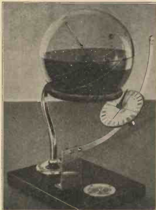
A front view of the Astroglobe with the quadrant arm shown on the right.
