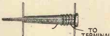
Fig. 2.—Details of the electro-magnet.
