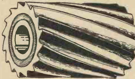
Fig. 9.—This type of cutter is known as a roller or cylindrical cutter
