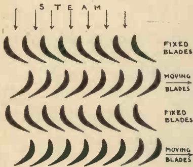
Fig. 2.—In addition to rotating blades there are stationary blades arranged in alternate rows to the rotating blades, as shown.
