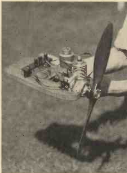
An American petrol engine mounted on a test block. It is fitted with a cast-iron liner, one ring, balanced crankshaft, rotary valve. It weighs, all on, 2 lb.
