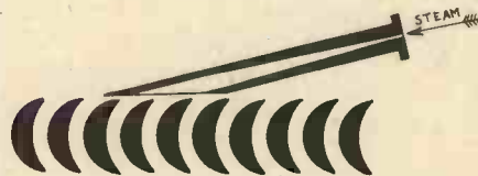
Fig. 1.—The principle of the De Laval turbine.
