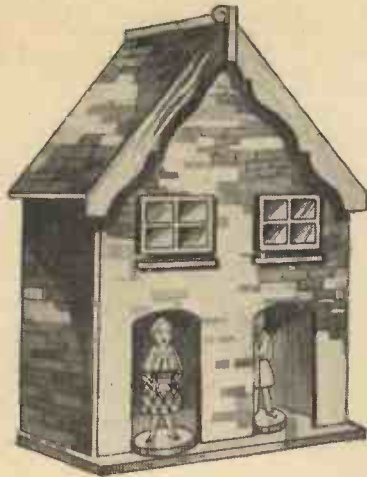
Fig. 1.—The finished weather cottage. The girl indicates fine and the man wet weather.
