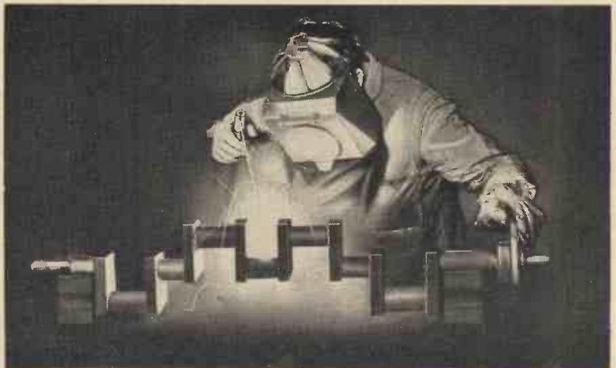
A trained engineer "flawless" electric-arc welding a crankshaft at the Barimar works.
