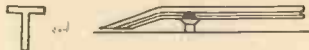
Figs. 6 and 7.—(Left) A section of the brass used for the jig shown in Fig. 5, and (right) the method of sloping off the conductor rail.
