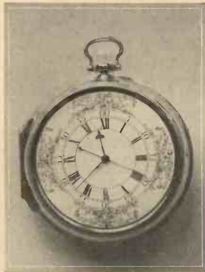
Figs. 4 and 5.—(Above) a front view of Harrison's fourth chronometer and (right) Harrison's second chronometer, 1739. This was the first to embody a "remontoire" mechanism for keeping a constant torque at the escape-wheel. It was never tested at sea because Britain was at war with Spain, but it was probably capable of winning the £10,000 reward.
