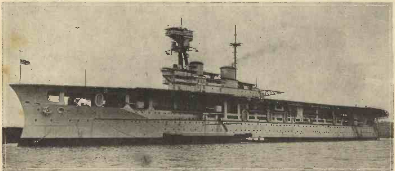
H.M.S. "Eagle" is a heavy boat, having a displacement of 25,000 tons, but although it is such a large vessel it can only accommodate 20 aircraft.
