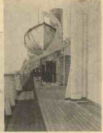
(From Left to Right). A view from the upper deck, showing the car park. The Swedish train ferry leaving Copenhagen Harbour for Malmö. A deck view, showing new patent davits which enable the boats to be launched even when there is a serious list on the ship.
