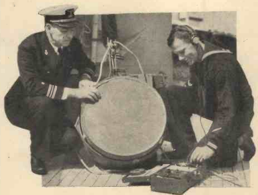
Showing the wireless operator and captain of a survey ship operating the hydrophone.
