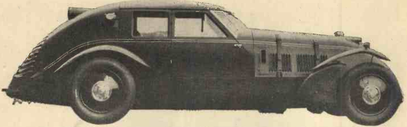
This impressive-looking saloon was built experimentally to test out the possibilities of the Diesel engine or high-speed purposes.
