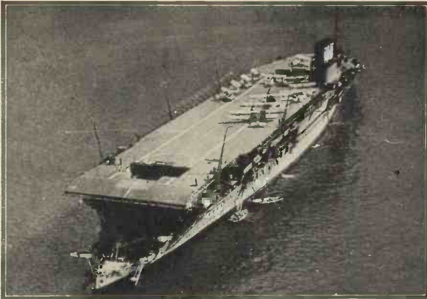
H.M.S. "Courageous," flagship of the aircraft carriers, photographed from the air with some of her machines arranged on deck. She carries a total of approximately 50 aircraft of three distinct types—fighters, torpedo bombers, and reconnaissance. These are raised and lowered into the hangars under the flight deck by lifts, both of which are down in this photograph, and the wells can be seen.
