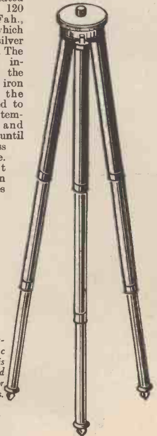
A tripod having telescopic legs, which is both rigid and adjustable for various heights.
