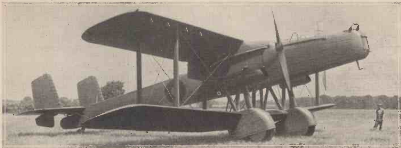
Fig. 1.—A side view of a Handley Page "Heyford." The cockpit is right up in the front fuselage, just behind the front gunner's cockpit.
