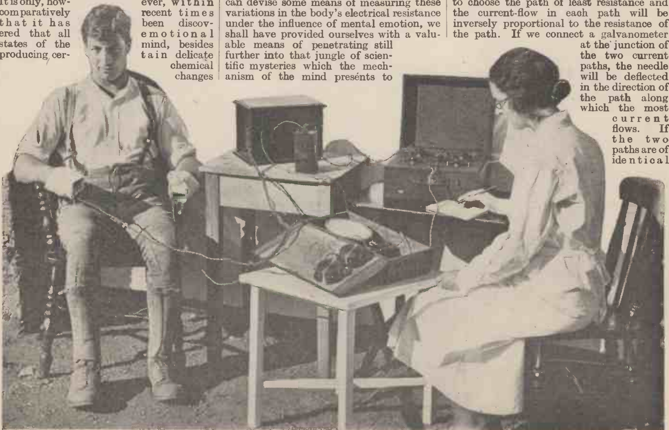
The lie machine in use. A subject being tested by means of psychogalvanic reflex apparatus.
