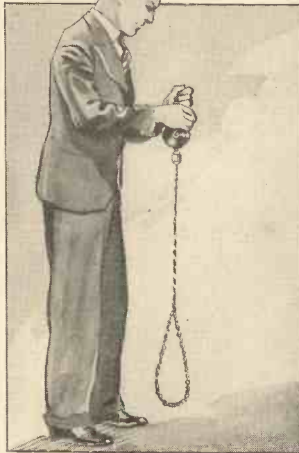
Fig. 1.—The chain held in the drill chuck ready for spinning.
