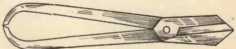
Fig. 22.—Tinmen's shears. A tool for cutting thin sheet metal and wire.
