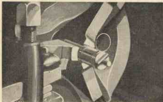
Fig. 6.—Adjusting the depth of the grooves.
