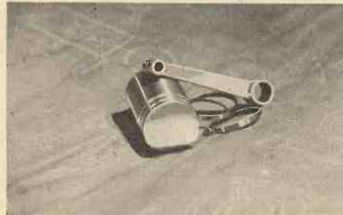
Fig. 7.—Showing the finished piston and connecting rod.
