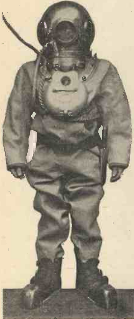
The closed diving dress introduced by Augustus Siebe in 1837. In this the diver was enabled for the first time to control the pressure of the air he breathed to suit the circumstances of his immersion.
