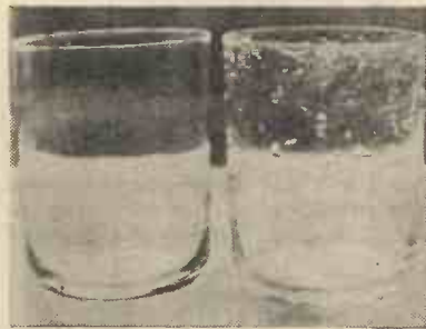
The glassware on the left is washed with water-glass, and on the right with washing soda. It will be seen that water-glass runs off cleanly.
