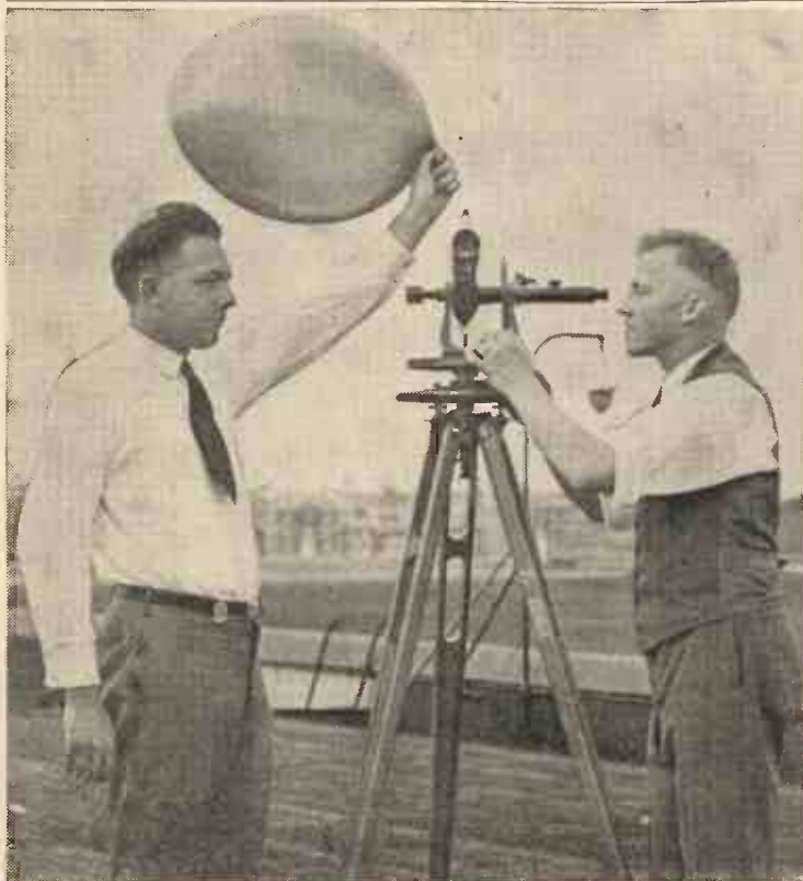
Testing the upper air conditions for the guidance of pilots.
