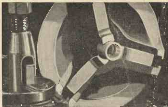
Fig. 5.—Scraping a small radius on the mouth of the piston before removing from the chuck.
