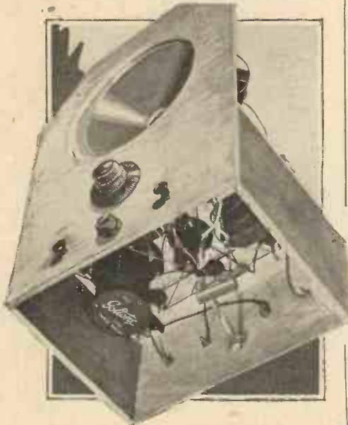
Showing the neat and compact arrangement of the components underneath the chassis.
