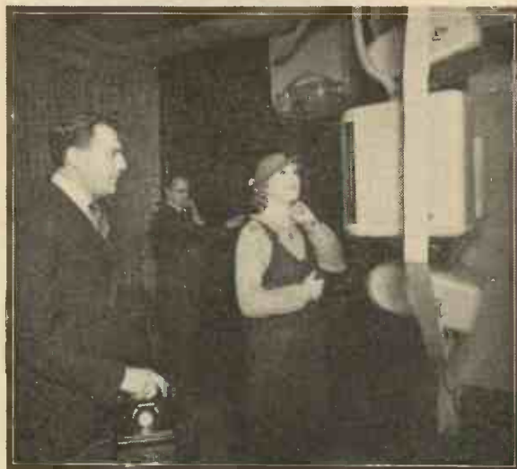
Fig. 6.—Showing how the photo-electric cells are arranged round the subject in the Baird light-spot studios.
