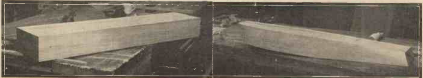
Two photographs showing how the hull is shaped from a solid block of wood.
