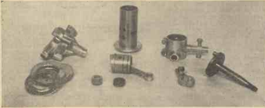
A complete set of machined parts for the Hallam 13.5 c.c. two-stroke petrol engine.
