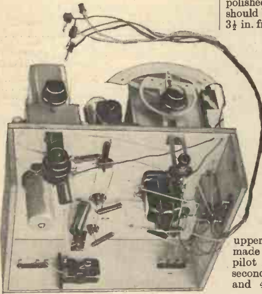
A photograph which shows the simplicity of the under-chassis wiring.
