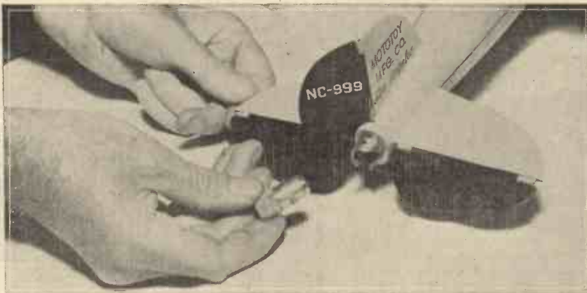
The tail unit of the model Lockheed Vega shown above. Note the power plug, which fits into the tail.
