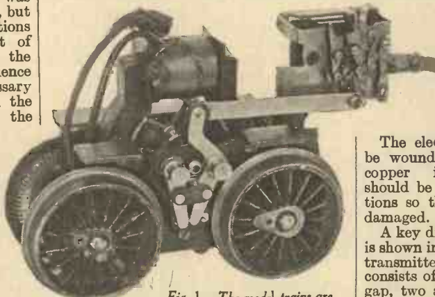
Fig. 1.—The model trains are fitted with "sequence" reversing mechanism as shown.
