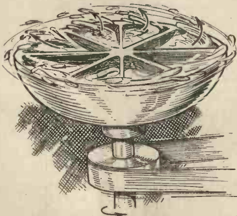
Fig. 2.—If the bowl is now rotating, oil will begin to fly upwards and outwards over the edge until the bowl is empty.
