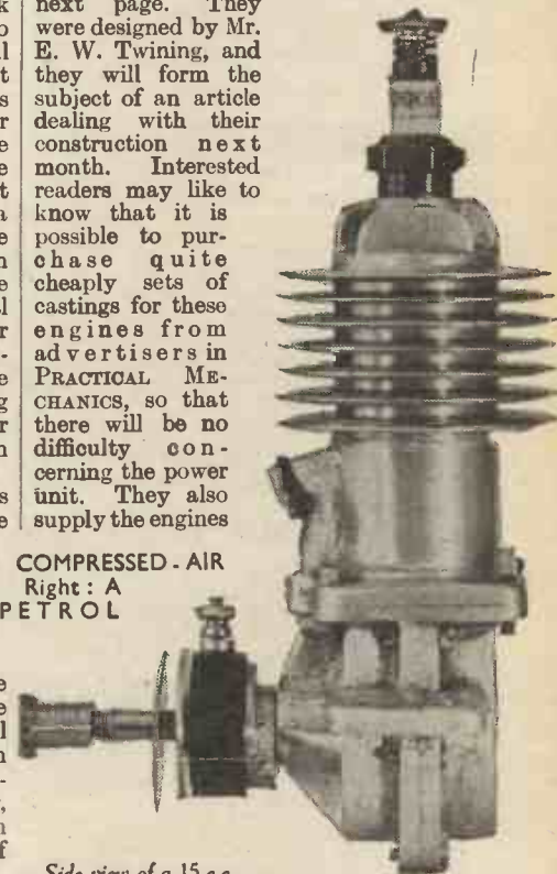
Side view of a 15 c.c. two-stroke model aeroplane engine made by the Author.
