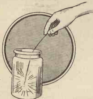
Fig. 3.—Here is another interesting experiment. Iron wire is made to spark by immersion in a jar of oxygen.
