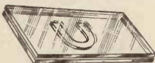
Fig. 4.—An easily-constructed device for viewing live objects in liquids. A small piece of "U"-shaped rubber is cemented between two plates of glass 2 in. long by 1 in. wide.
