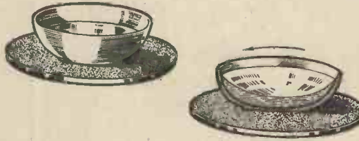
Fig. 1.—On the left is a bowl of oil. On the right the same bowl being spun round. The liquid takes up the position shown. This is the germ of the fluid flywheel in its simplest form.
