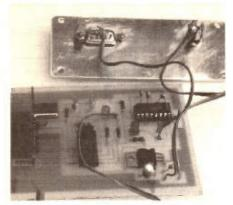
Wiring from the p.c.b. to the D-type connector and the power socket on the rear panel.
