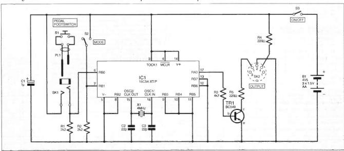
Fig.3. Full circuit diagram for the PIC MIDI Sustain Pedal.
