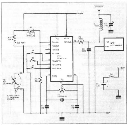
Fig.4. Complete circuit diagram for the Transmitter. Note that switches S1 to S4 are d.i.l. slide types.
