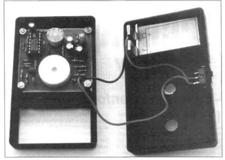
Wiring between the two halves of the completed Alarm case. The p.c.b. is situated in the section which takes the battery cover. Note the siting of the On/Off slide switch on the side of the case.
