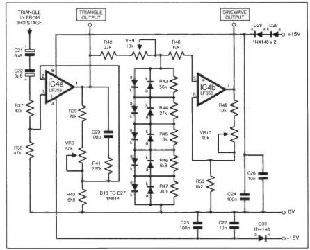
Fig.4d. Circuit diagram for the Buffer stage.
