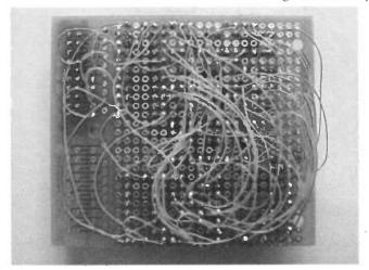
Underside wiring for the 8-bit interrupt latch.
