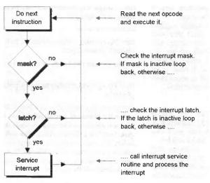
Fig.3. Interrupts handling flow-chart.
