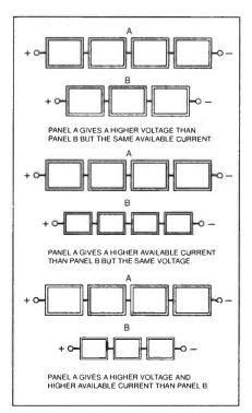
Different power and voltage configurations with solar cells.
