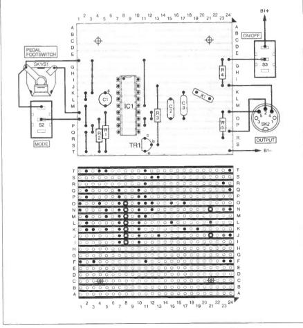
Fig.4. Stripboard topside component layout, interwiring to off-board components and underside view of the copper tracks showing locations of breaks required in the strips.
