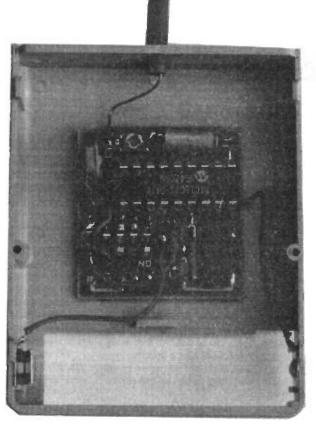
Positioning of the p.c.b. inside the Transmitter case.
