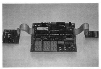
The interrupt latch and l.e.d. output modules connected to PhizzyB.
