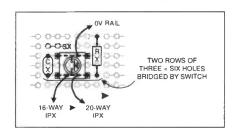
Fig.2. Switch wiring details.
