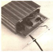
Slotting the p.c.b. into the case.
