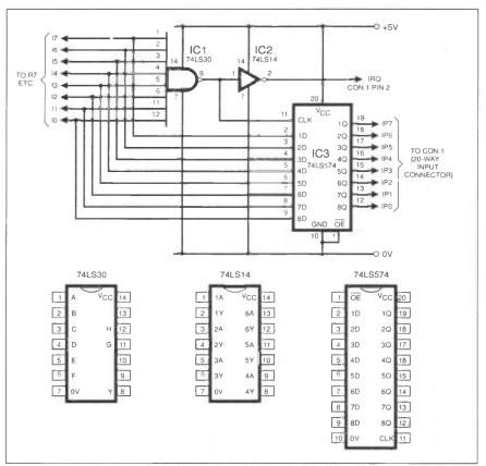
Fig.3(a). Basic circuit diagram of the 8-bit latch and (b) the pinouts of the associated
