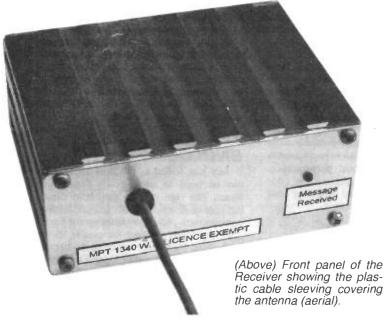
sarily require an internal battery compartment. If required, the unit can be powered from any supply between 3V and 6V d.c. Do bear in mind, though, that a high capacity cell is required if the particular application demands that the unit be switched on for long periods at a time.
