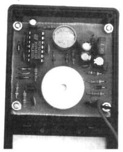
Circuit board bolted into the lower half of the case.
