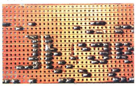
Solder bridges are most likely to occur where joints are tightly packed, especially around d.i.l. integrated circuits. The larger solder blob is a type that should be instantly spotted and rectified. The smaller one at the bottom left-hand corner of the cluster is less obvious, but should soon be spotted when giving the board a careful inspection with an "eyeglass".
