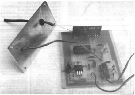
The r.f. status l.e.d. mounted and wired on the front panel. This can also be accompanied by the RS232 com status I.e.d. if preferred.
