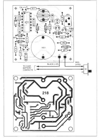
Fig.2. Light Alarm printed circuit board component layout, full-size copper foil master and wiring to the battery connector and On/Off slide switch.
