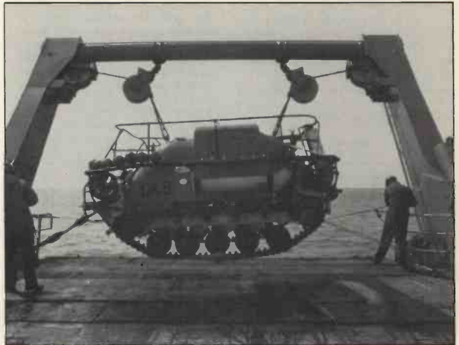
Submersible cable trencher "Sea-Dog" being lowered. Reproduced by kind permission of British Telecom.
