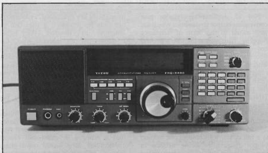
The YAESU FRG-8800. Its synthesiser and up-converter technique give continuous tuning from 150 kHz to 30MHz (plus keyboard tuning and automatic scanning).
