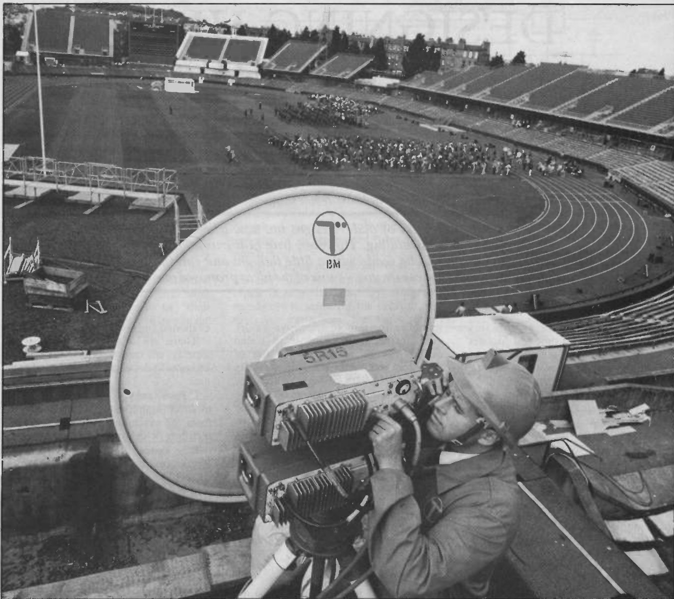
Photo.1. Shows a B.T. engineer making final adjustments to the microwave dish which carried broadcast transmissions of the opening ceremonies of the 1986 Commonwealth Games.
