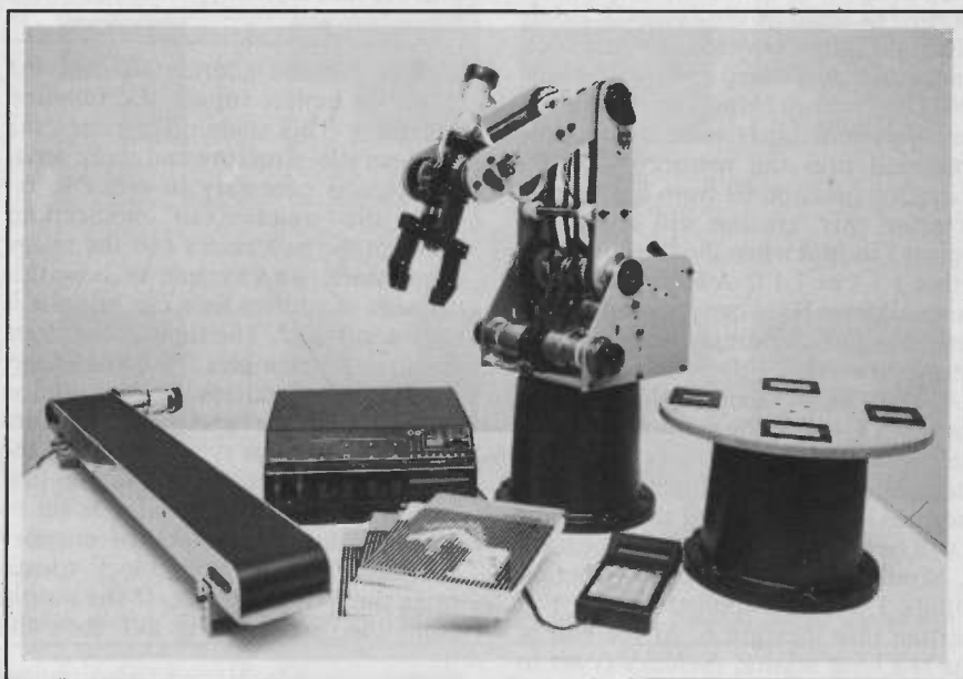
Photo 1. Scorbot ER III rotary table and conveyor
