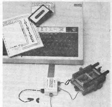
The Pilot One Buggy Controller linked to a BBC micro and a Lego model kit
