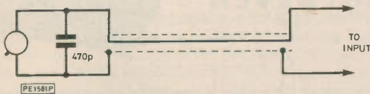
Fig. 2.16. Input arrangement for ceramic pick-up cartridges
