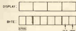
Fig. 4. The assignment of bits to Life patterns in the program of Fig. 5.
