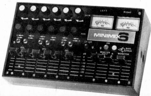
This is done by closing the monitoring switch on the input channel in question and also by changing over the input/output monitor switch. In these circumstances the input signal is routed to both meter and monitoring amplifiers.
