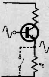
Fig. 3.4. The divider to feed base bias is irrelevant to this circuit which demonstrates the effect of R_E
