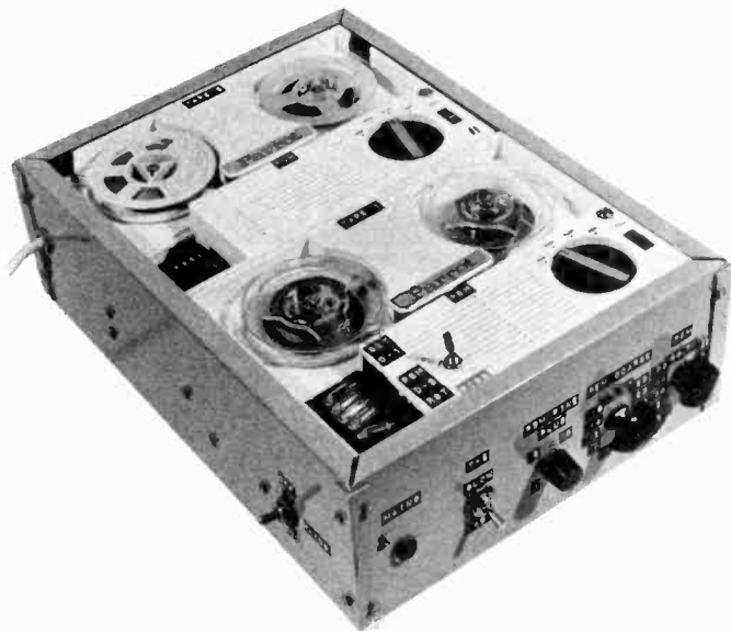
The completed Callercord showing the two Parrot recorders in position. These are simply supported on angle strips. Note the siting of the neon display panel and call counter which occupy the space normally taken by the microphones
