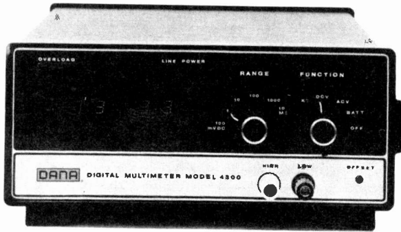
The large L.E.D. devices used in this instrument are automatically varied in brightness by ambient light conditions (Dana)
