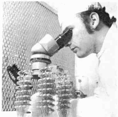
Transistor "headers" being examined for flaws
