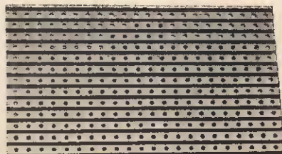
Fig. 2a. Underside view of Veroboard showing the copper strips
