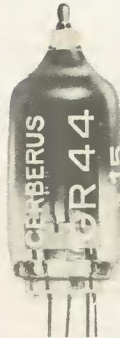
The Cerberus GR44 trigger tube; this tube has twin trigger electrodes and a priming anode
