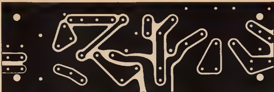
Fig. 2. Printed circuit pattern for cymbals filter (full size)
