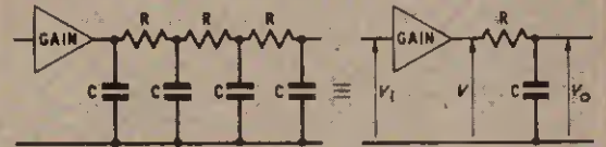
Fig. 4.12. Equivalent circuit of a transistor looks like that of a transmission line at high frequencies
