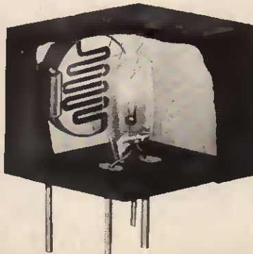
Photo-cell lamp assembly marketed by Hird-Brown
