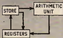
Fig. 5.2. Add an arithmetic unit
