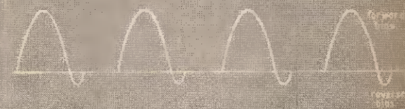
Fig. 1b. Current through a typical semiconductor diode
