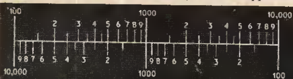
Fig. 1. Inversion chart for finding the combined value of two resistances in parallel
