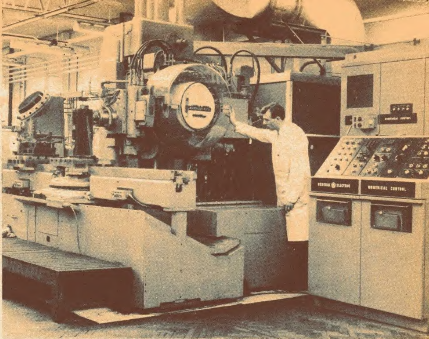
Fig. 4. One of three numerically controlled Milwaukee-Matic machines in operation at I.C.T.'s Stevenage factory. A control tape produced by an I.C.T. computer is used to govern the operation of the machine tools to produce castings for further I.C.T. computer systems
