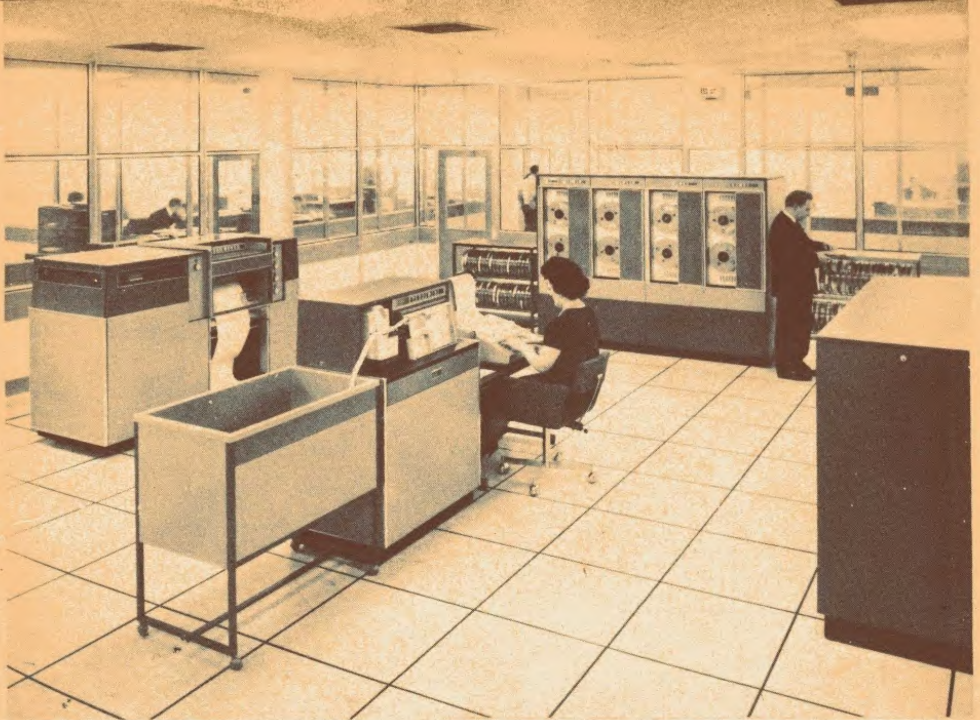
Fig. 2. An I.C.T. 1903 computer system recently installed at English Sewing Cotton Co. Ltd., Manchester. The picture shows, from left to right, a line printer, paper tape reader, console typewriter, magnetic tape storage units and central processor
