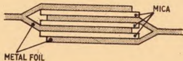
Fig. 5.4. Alternate layers of mica and metal foil are stacked in this manner to form a capacitor
