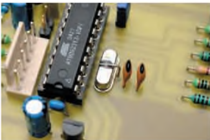
This close-up view shows how a wire link is used to connect the crystal case to a ground pad.
