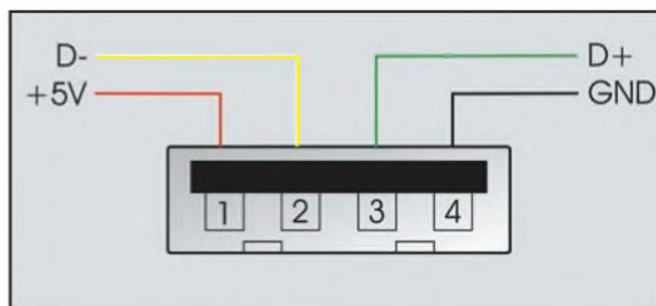
Fig.1. PCs are master devices that have a type A USB socket. Communication is via a three-wire link, with a fourth wire providing a +5-volt supply
