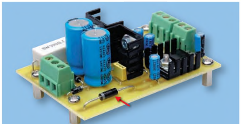
Replace the 100 \Omega 5W resistor on the power supply board with a 5.1V 5W Zener diode, as shown here. Note the orientation of the cathode (banded) end of the Zener.
